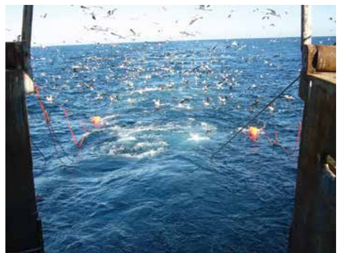
Tori/bird scaring lines deployed behind fishing vessel. Photo: Barry Watkins, BirdLife Albatross Task Force, South Africa.
